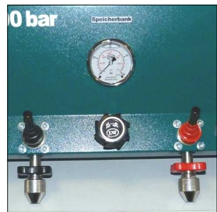
Fig. 1 - Hand wheel valve and pressure gauge
