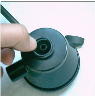
Fig. 4 - Place o-ring into the groove
