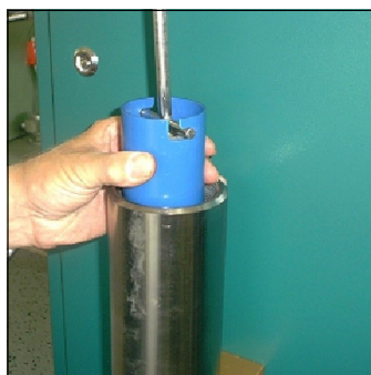
Fig. 4 - Pull the cartridge out of the housing.
