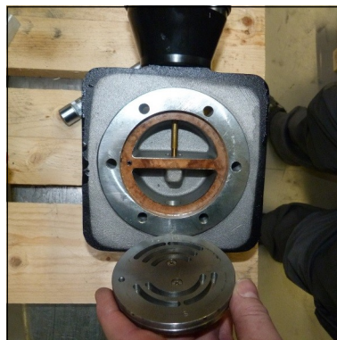
Fig. 2 - Remove in- and outlet valve
