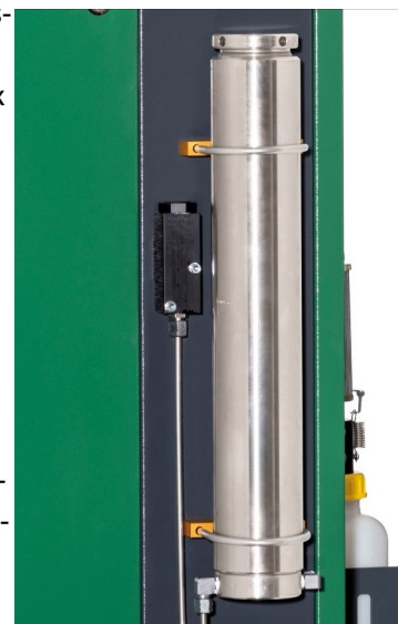
Oil / water separators final stage
