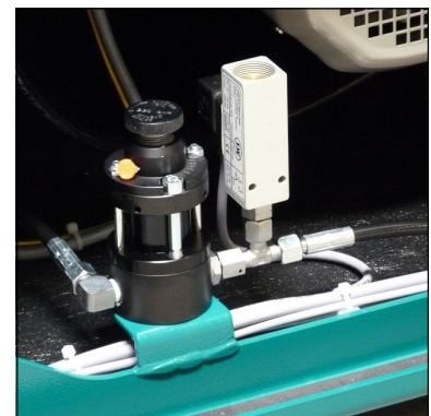
Safety valve 3rd stage
