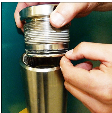
Fig. 2 - Change o-ring and back-up rings
