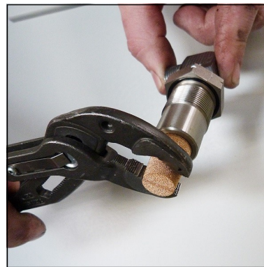
Fig. 3 - Change sinter filter
