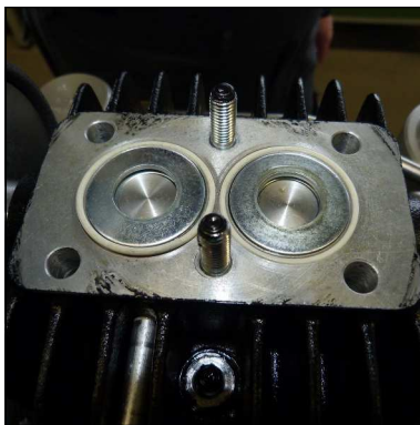
Abb. 5 - Federteller in Ventilkopf
