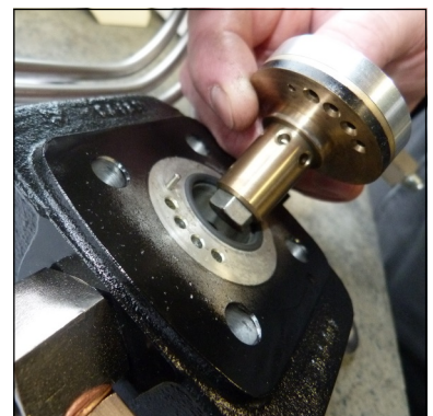
Fig. 4 - Ensure correct valve position (centre pin)
