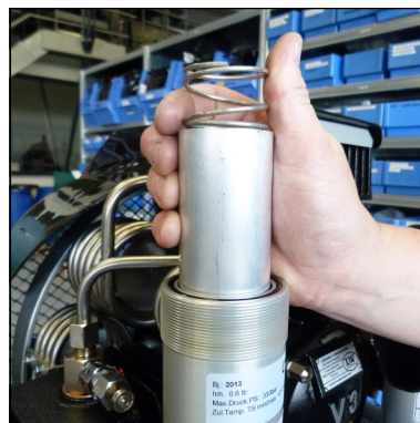
Abb. 2 - Remove filter cartridge
