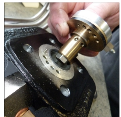
Fig. 5 - Ensure correct valve position (centre pin)
