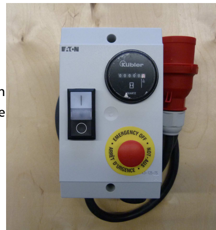
Remote control box c/w hour counter
