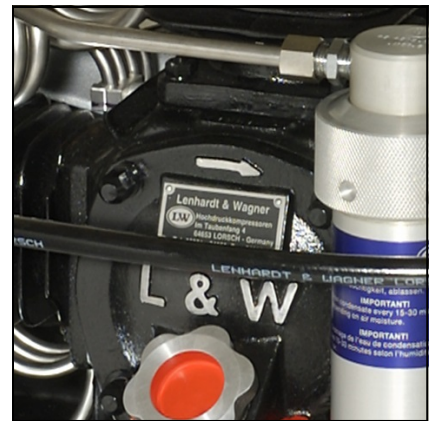
Rotation direction arrow on the compressor block
