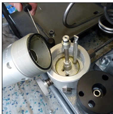
Abb. 4 - Remove lock ring
