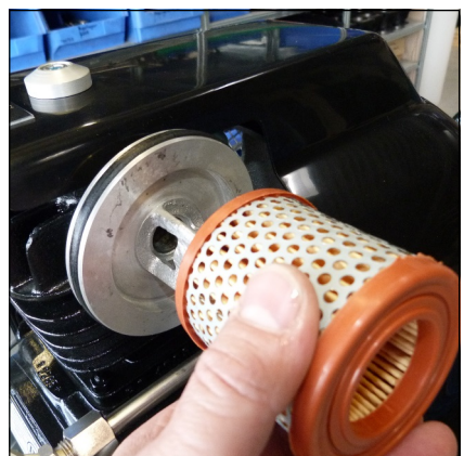
Fig. 3 - Change intake filter
