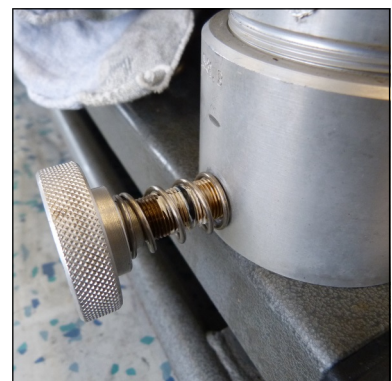
Abb. 6 - O-ring, condensate drain valve
