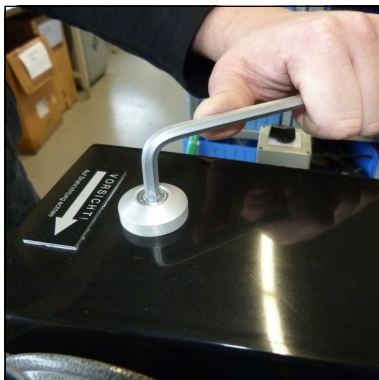
Fig. 1 - Remove top mounting screws
