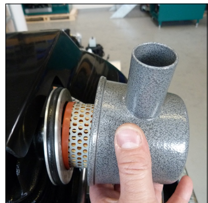
Fig. 2 - Remove intake filter housing cover
