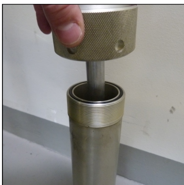
Abb. 4 - Remove lock ring and change o-ring
