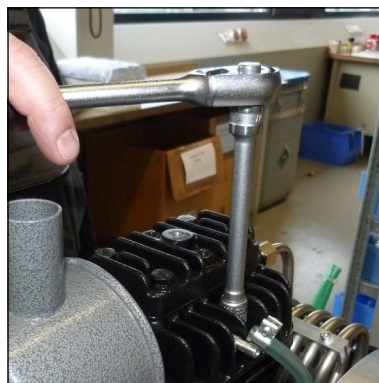
Fig. 6 - Tighten valve head
