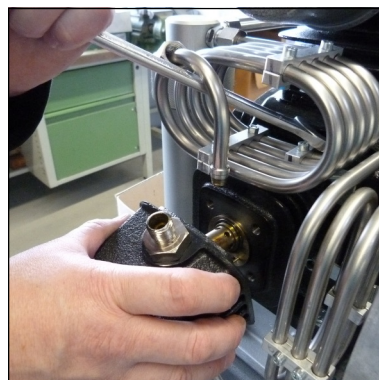
Fig. 3 - Remove valve head
