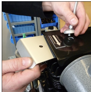
Fig. 2 - Remove protection plate
