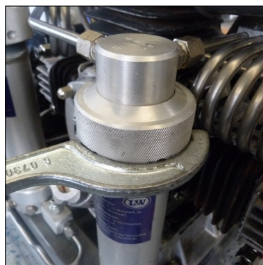
Abb. 5 - Tighten lock ring
