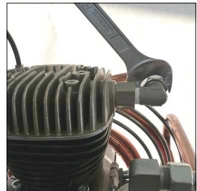
Fig. 6 - Connect pipe connections and tighten
