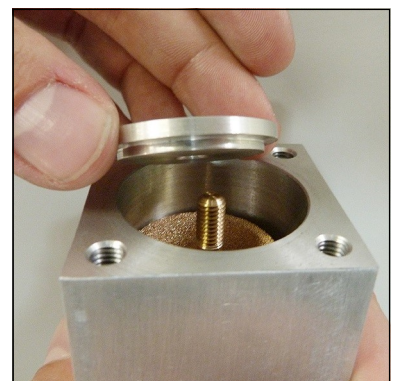
Fig. 5 - Place filter washer and washer
