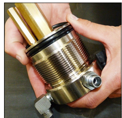
Fig. 4 - Change o-ring and back-up rings
