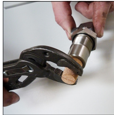
Fig. 3 - Change sinter filter
