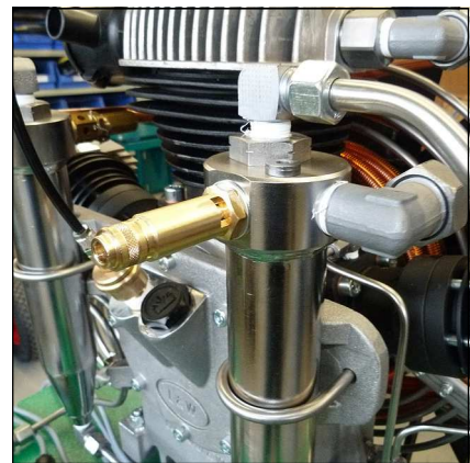
Safety valve 1st stage
