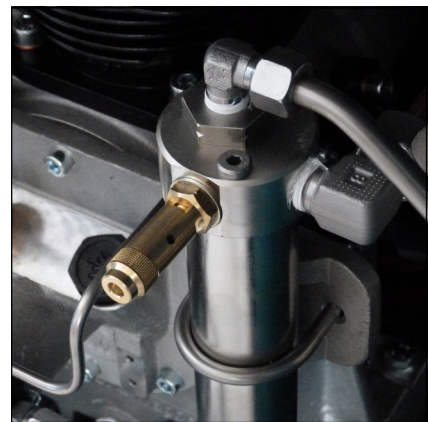
Safety valve 1st stage
