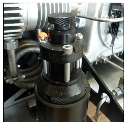
Fig. - Safety valve 3rd stage
