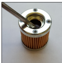
View bypass valve
