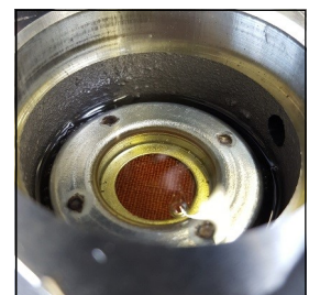
Installation view oil filter
