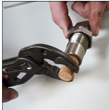
Fig. 3 - Change sinter filter
