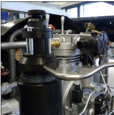
Fig. 1 - Loosen filter housing topcap by using the filter tool
