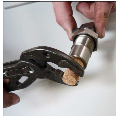
Fig. 3 - Change sinter filter
