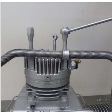
Fig. 5 - Remove cooling pipe bracket
