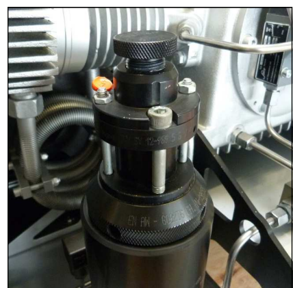
Fig. - Safety valve 3rd stage
