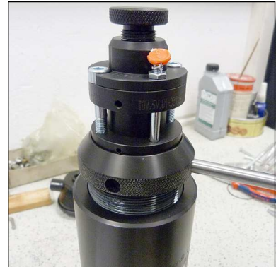
Fig. 1 - Remove/screw in filter cover
