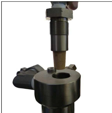
Fig. 2 - Remove sinter filter holder
