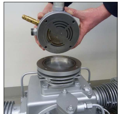
Fig. 7 - Remove valve head
