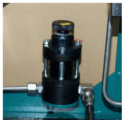
Safety valve 3rd stage
