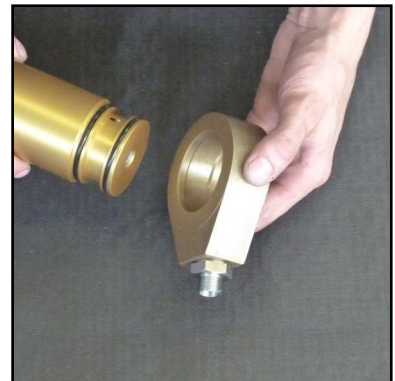
Abb. 6 - Remove the base ring
