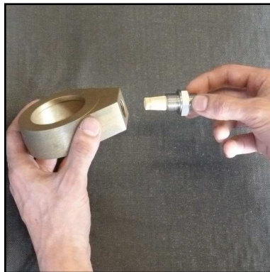
Abb. 7 - Change sinter filter
