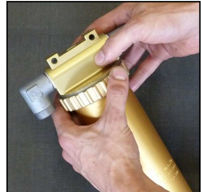
Fig. 1 - Open ring nut and remove separator top
