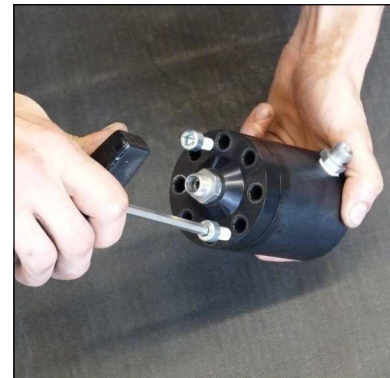
Fig. 2 - Remove the cover
