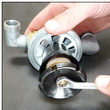
Fig. 2 - Loosen nut at the separator top
