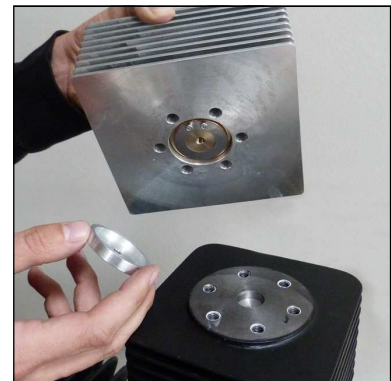
Fig. 2 - Remove lower valve gasket
