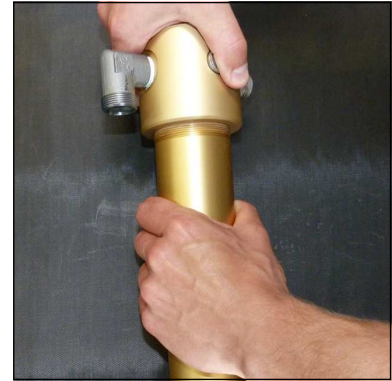
Fig. 1 - Unscrew and remove filter top
