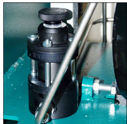
Safety valve 3rd stage
