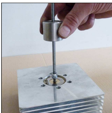
Fig. 3 - Remove inlet and outlet valve
