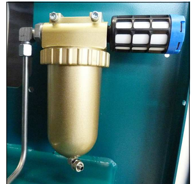
Oil / water separators final stage
