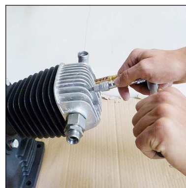
Fig. 1 - Loosen valve head screws
