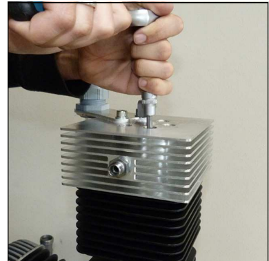
Fig. 1 - Loosen valve head screws
