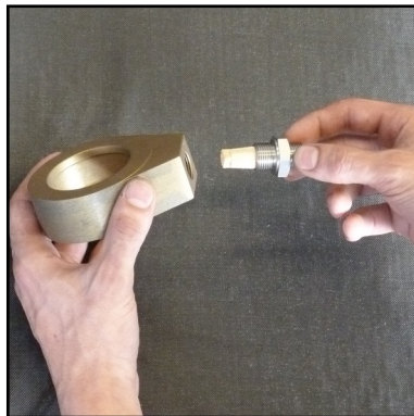
Abb. 7 - Change sinter filter
