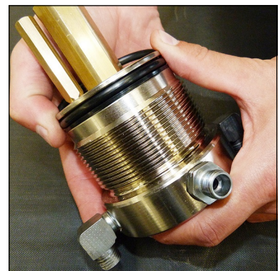
Fig. 4 - Change o-ring and back-up rings
