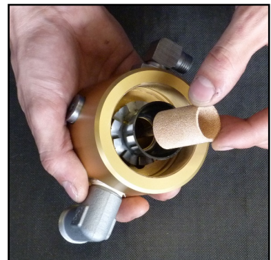
Fig. 3 - Change sinter filter
