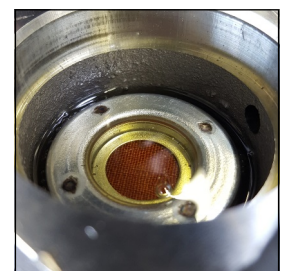
Installation view oil filter
