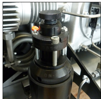
Fig. - Safety valve 3rd stage
