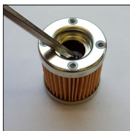
View bypass valve
