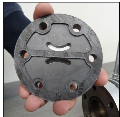
Fig. 2 - Correct mounting position of upper valve gasket
