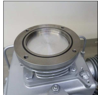
Fig. 1 - Change lower gasket (o-ring)
