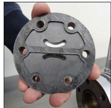
Fig. 2 - Correct mounting position of upper valve gasket
