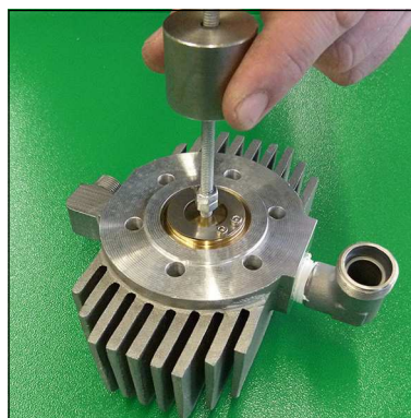
Fig. 4 - Remove inlet and outlet valve
