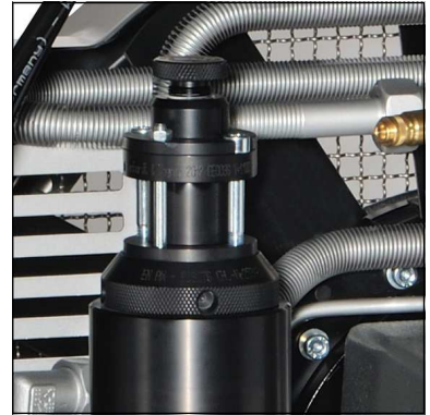
Fig. 1 - Remove/screw in filter cover
