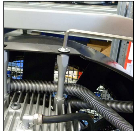
Fig. 1 - Remove top mounting screws
