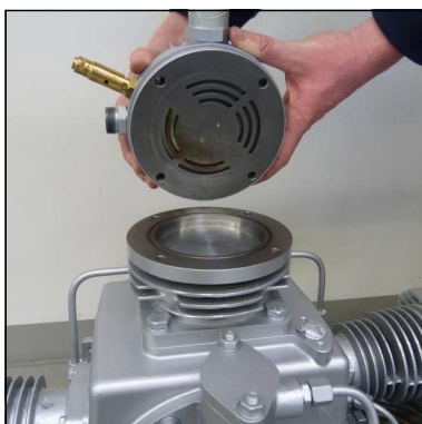
Fig. 3 - Place valve head to cylinder
