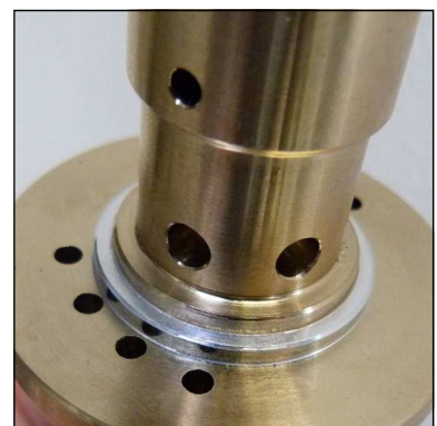
Fig. 5 - Ensure correct mounting position of the upper valve gasket
