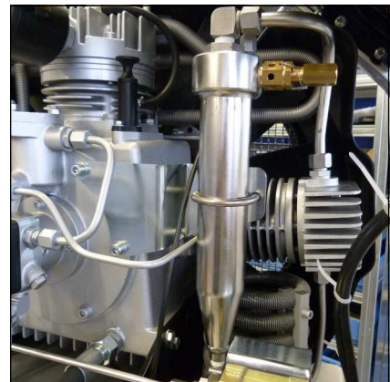
Oil / water separators 2nd stage
