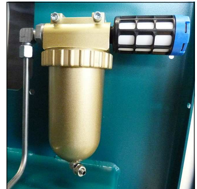
Oil / water separators final stage
