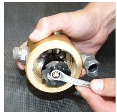
Fig. 2 - Loosen nut at the separator top
