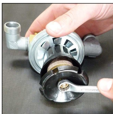
Fig. 2 - Loosen nut at the separator top
