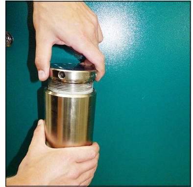
Fig. 1 - Open Filter cover
