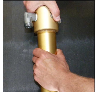
Fig. 1 - Unscrew and remove filter top
