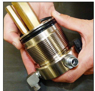
Fig. 4 - Change o-ring and back-up rings
