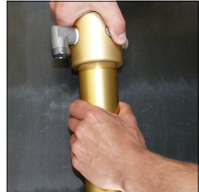
Fig. 1 - Unscrew and remove filter top
