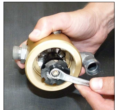
Fig. 2 - Loosen nut at the separator top
