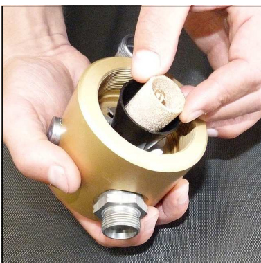
Fig. 3 - Change sinter filter
