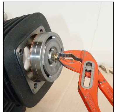
Fig. 2 - Pull out inlet and outlet valve
