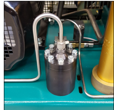
Fig. 1 - Condensate stop valve housing
