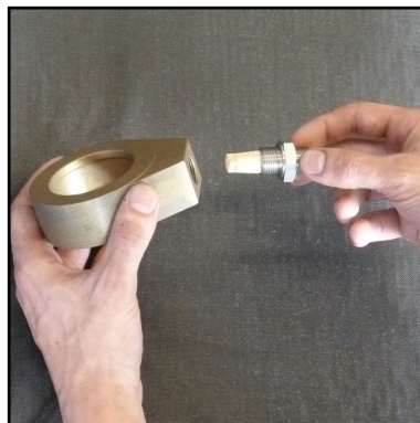
Abb. 8 - Change sinter filter
