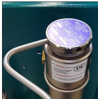
Fig. 2 - Unscrew the filter housing cover.
