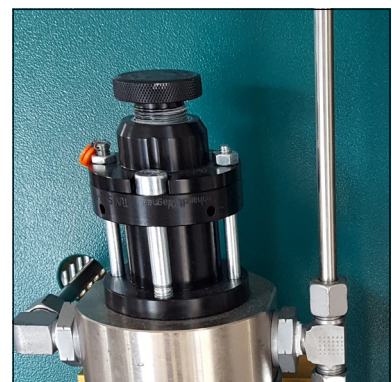
Safety valve 4th stage
