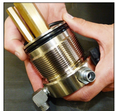
Fig. 4 - Change o-ring and back-up rings
