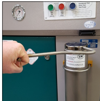
Fig. 2 - Unscrew the filter housing cover.
