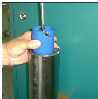
Fig. 4 - Pull the cartridge out of the housing.
