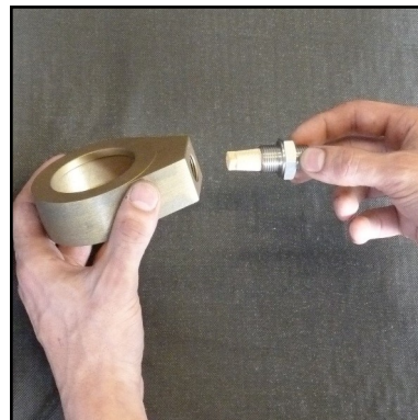
Abb. 8 - Change sinter filter
