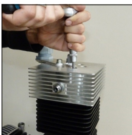
Fig. 1 - Loose valve head screws
