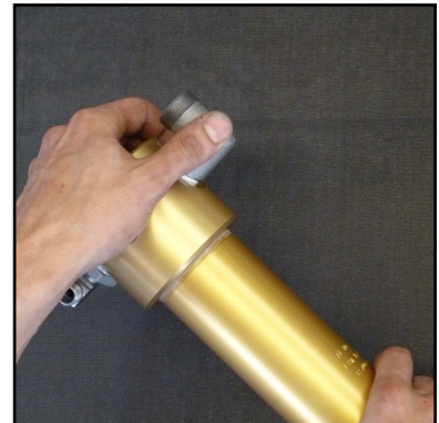
Fig. 1 - Unscrew and remove filter top
