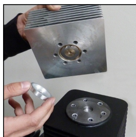
Fig. 2 - Remove lower valve gasket
