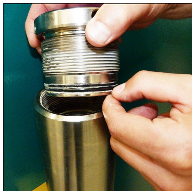
Fig. 2 - Change o-ring and back-up rings
