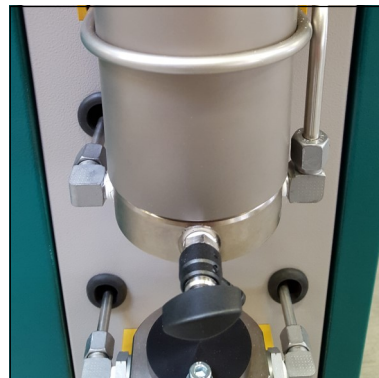
Fig. 3 - Loose pipe connections and nuts
