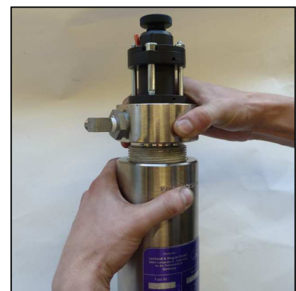
Fig. 3 - Open pre-filter cover
