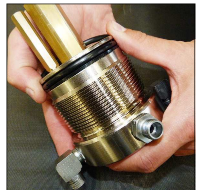
Fig. 4 - Change o-ring and back-up rings
