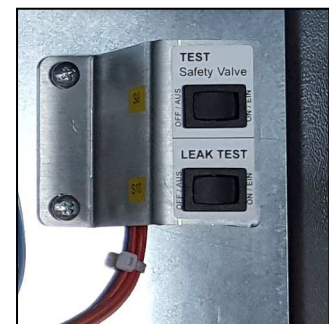
Leak test switch (down)
