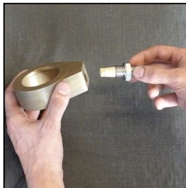
Abb. 8 - Change sinter filter
