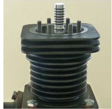
Fig. 1 - take off compression cylinder
