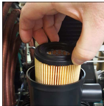
(Fig.2) Remove cover and replace filter cartridge
