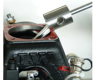
Fig. 2 - Piston 3rd Stage
