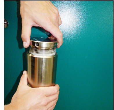
Fig. 1 - Open Filter cover
