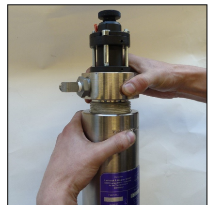
Fig. 3 - Open filter cover
