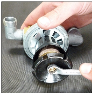
Fig. 2 - Loosen nut at the separator top
