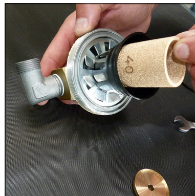
Fig. 3 - Change sinter filter
