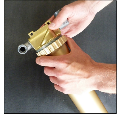
Fig. 1 - Open ring nut and remove separator top
