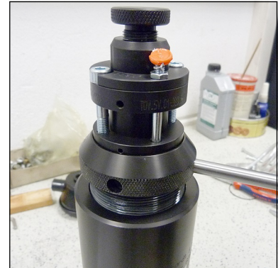
Fig. 1 - Remove/screw in filter cover
