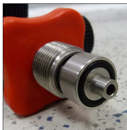
Fig. 1 - O-ring at the filling valve
