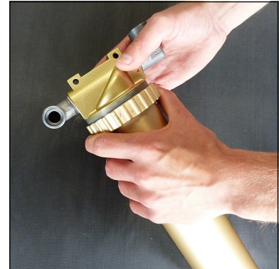
Fig. 1 - Open ring nut and remove separator top
