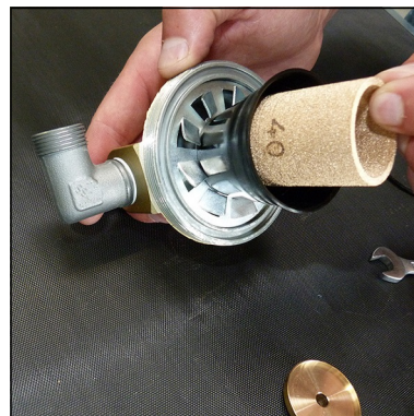
Fig. 3 - Change sinter filter
