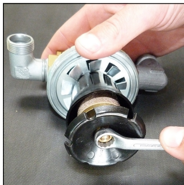
Fig. 2 - Loosen nut at the separator top
