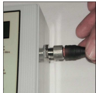
Connect cable (4 - 20 mA) to the control unit
