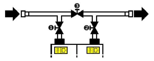
**CAUTION! Damage by pressure shocks!** The exposure with pressure of the refrigerant compressed air dryer has to happen slowly. The valve operations must necessarily be done slowly to avoid pressure shock.
