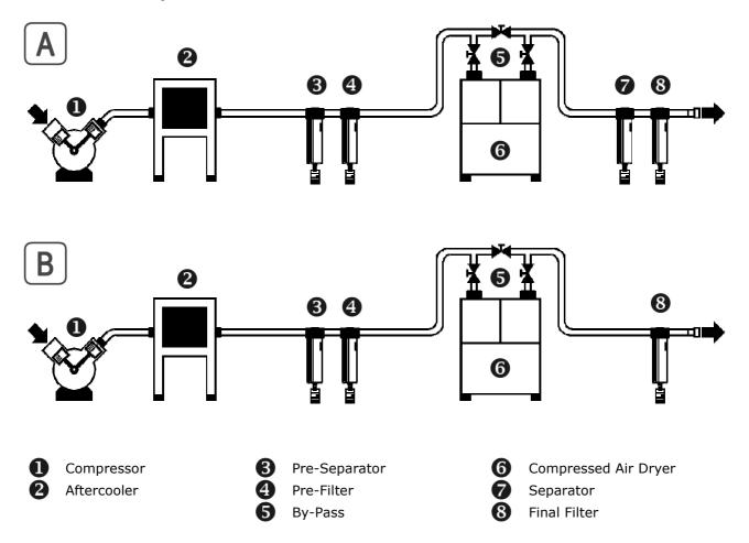
**Type A** installation with downstream separator (and mechanically operated venting unit) is suggested for dryer model "BASIC". **Type B** installation is suggested for dryer model "ACD which is already equipped with a built-in separator and condensate drain.
