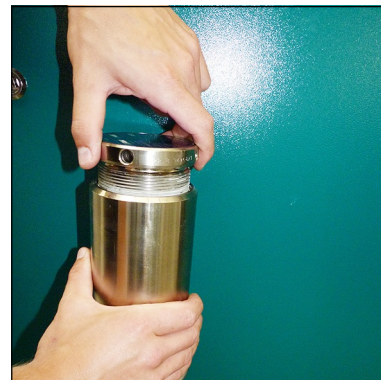
Fig. 1 - Open Filter cover
