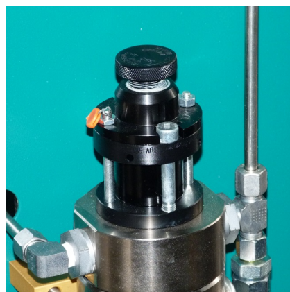
Safety valve 3rd stage
