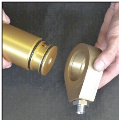
Abb. 5 - Remove the base ring
