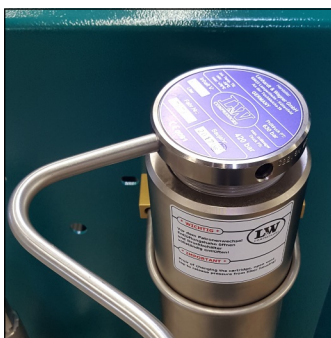
Fig. 2 - Unscrew the filter housing cover.
