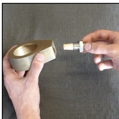
Abb. 7 - Change sinter filter
