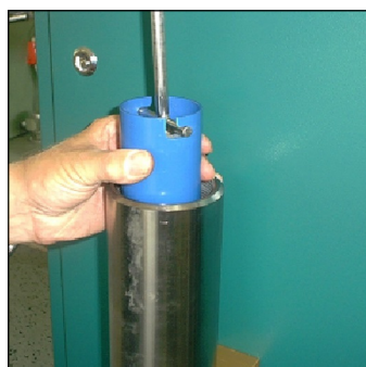
Fig. 4 - Pull the cartridge out of the housing.
