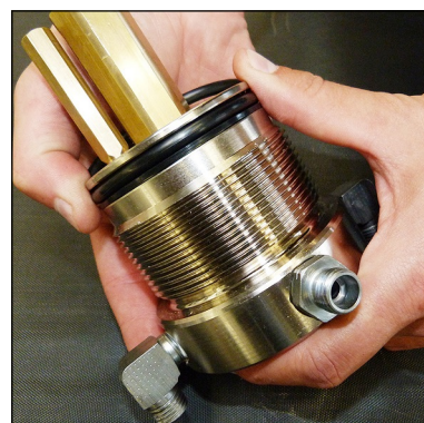
Fig. 4 - Change o-ring and back-up rings
