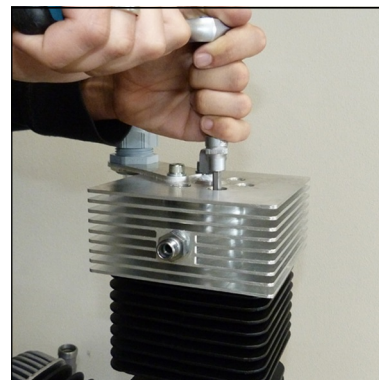
Fig. 1 - Loosen valve head screws
