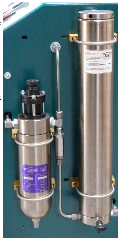
Filterhousing 1.7l (right), and filter unit 0,8l with safety valve (left)
