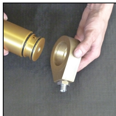
Abb. 6 - Remove the base ring
