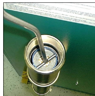
Fig. 3 - Place the T-piece end of the filter key in the top of the filter cartridge.
