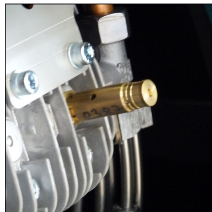
Safety valve 2nd stage
