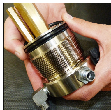
Fig. 4 - Change o-ring and back-up rings
