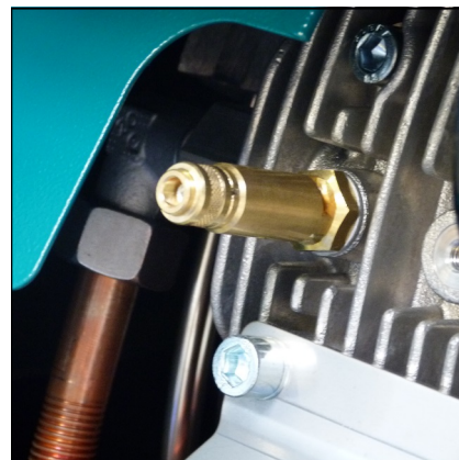
Safety valve 1st stage
