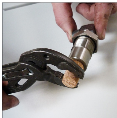
Fig. 3 - Change sinter filter
