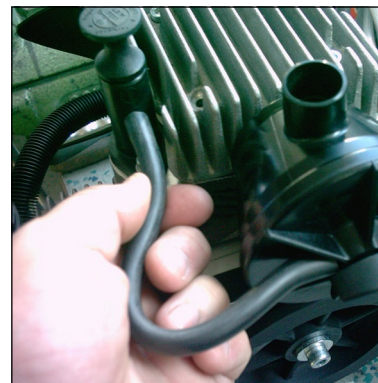
Fig. 6 - Connect ventilation hose at the oil fill port
