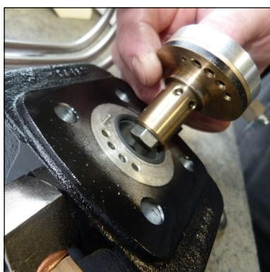
Fig. 1 - Ensure correct valve position (centre pin)
