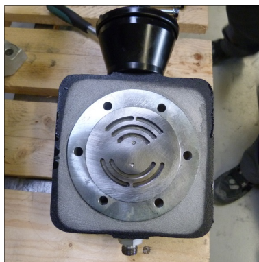
Fig. 3 - Correct position of in-and outlet valve
