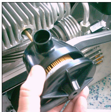
Fig. 2 - Pull out filter housing carefully
