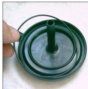
Fig. 3 - Place o-ring into the filter housing
