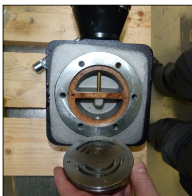
Fig. 2 - Remove in- and outlet valve
