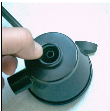
Fig. 4 - Place o-ring into the groove
